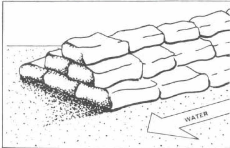
Figure 10: Stacking Sandbags in a Pyramid
